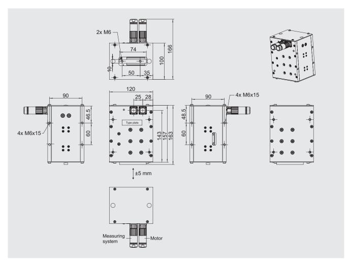
**LDDS-032-C**System data, system components, motor data
