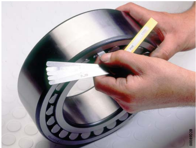
Figure 11 Measuring the radial internal clearance
